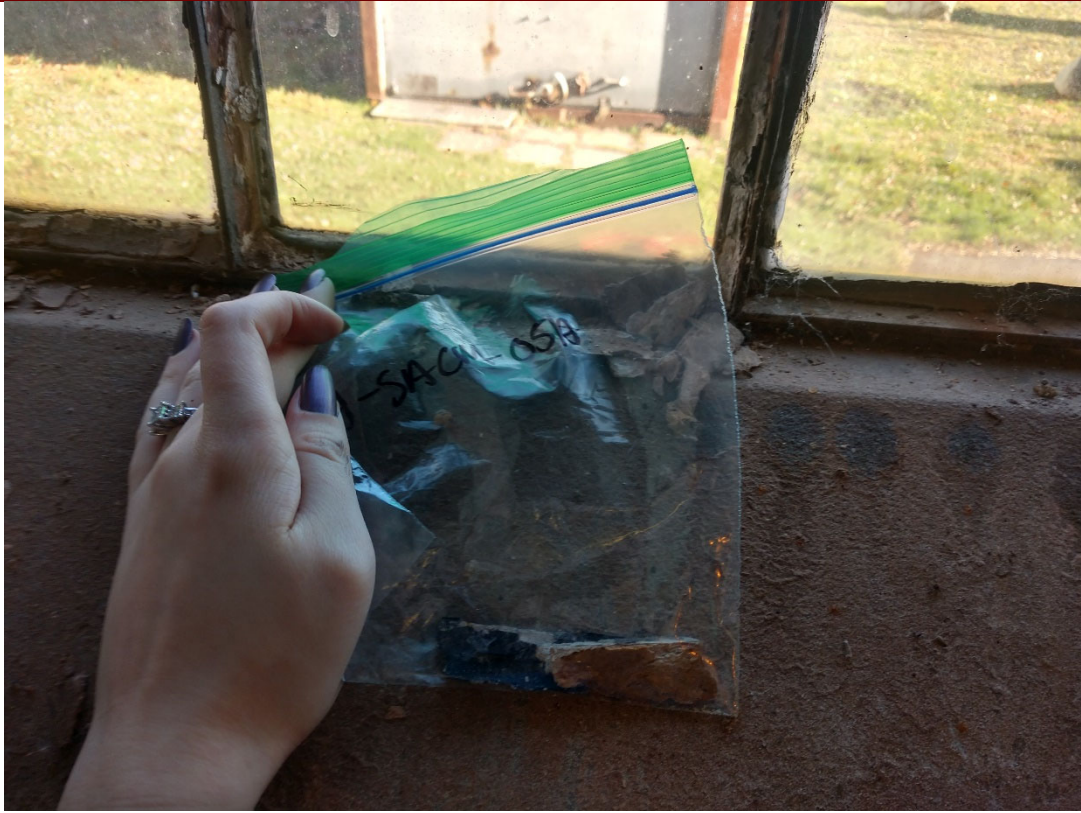
5. Material CA-SACM-05, off-white glazing found on the original building windows
