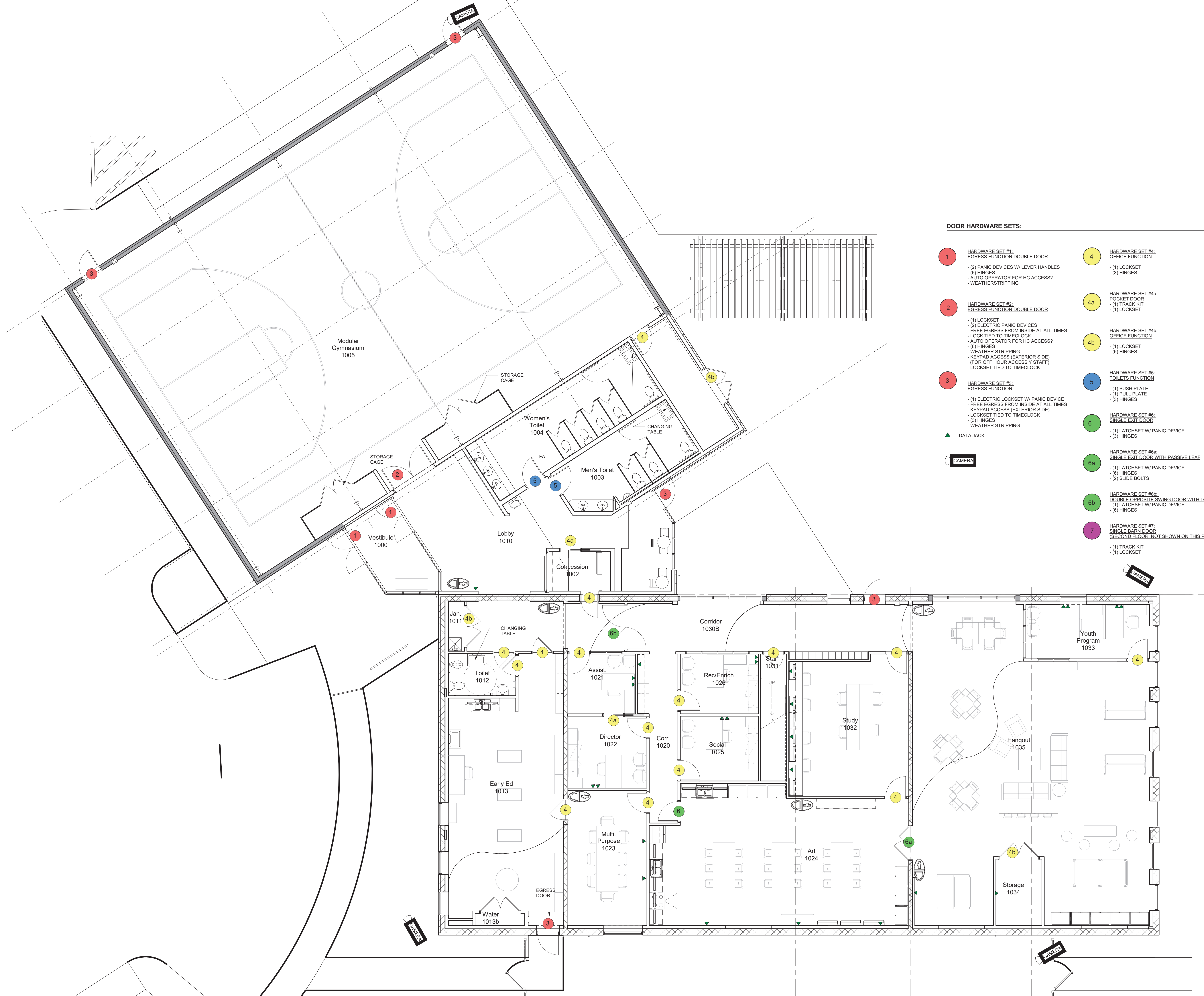
1 Door Hardware Diagram 3/16" = 1'-0"
