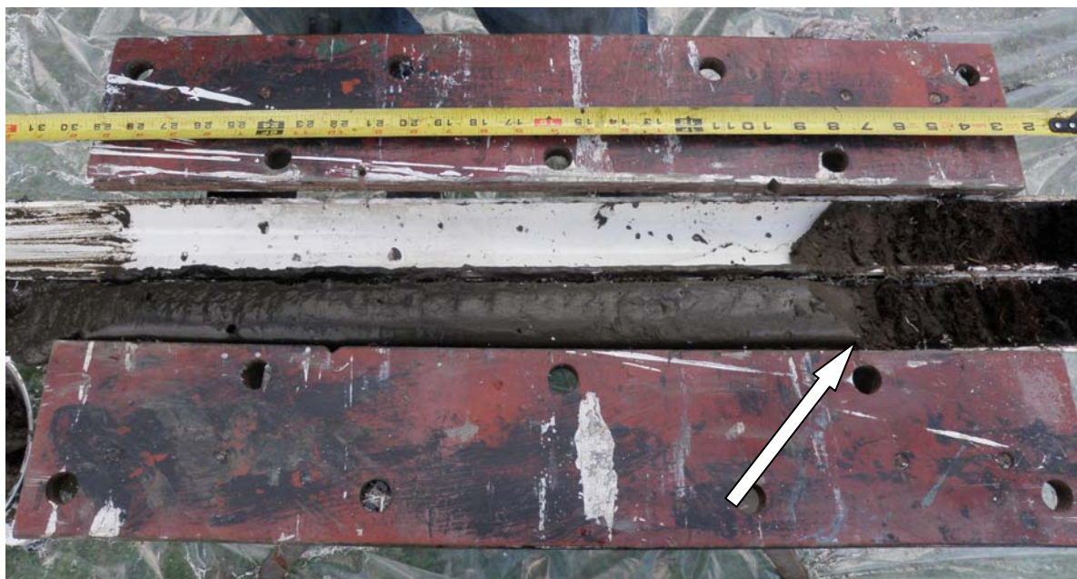
Photo 1. Sediment core sample 2 after cutting the PVC tube open, note transition from gray organic silt to dark brown peat.
