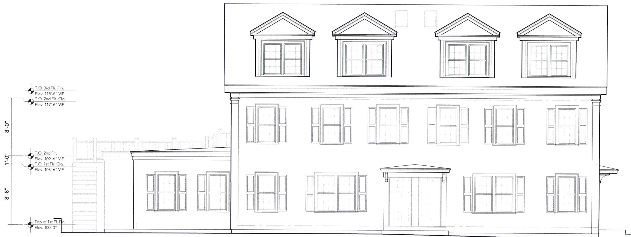
2 Side Exterior Elevation - BROAD STREET SCALE: 1/8" = 1'-0"
