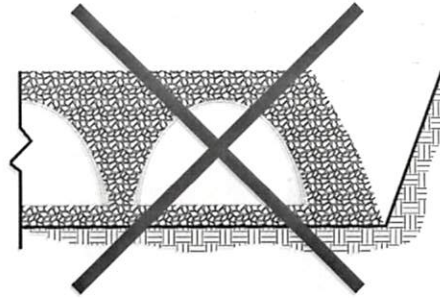
PERIMETER NOT BACKFILLED
