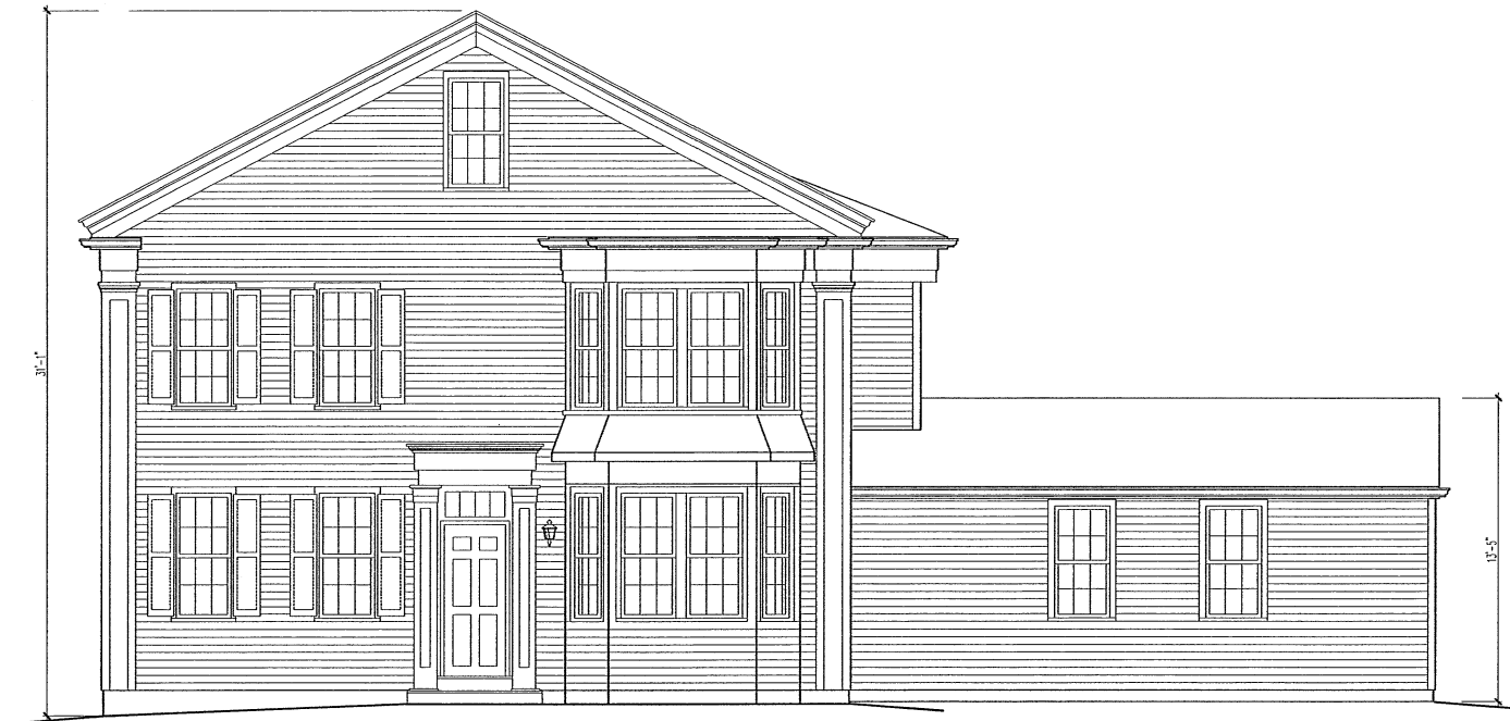
EXISTING RIGHT SIDE ELEVATION
