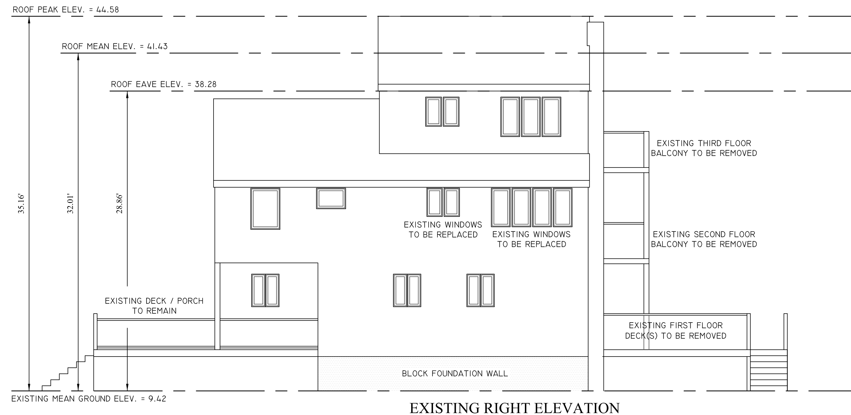
EXISTING RIGHT ELEVATION
