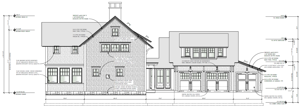
Figure 40 – Front Elevation (looking west) of the Proposed Single Family House on Lot 2 off Union Street
