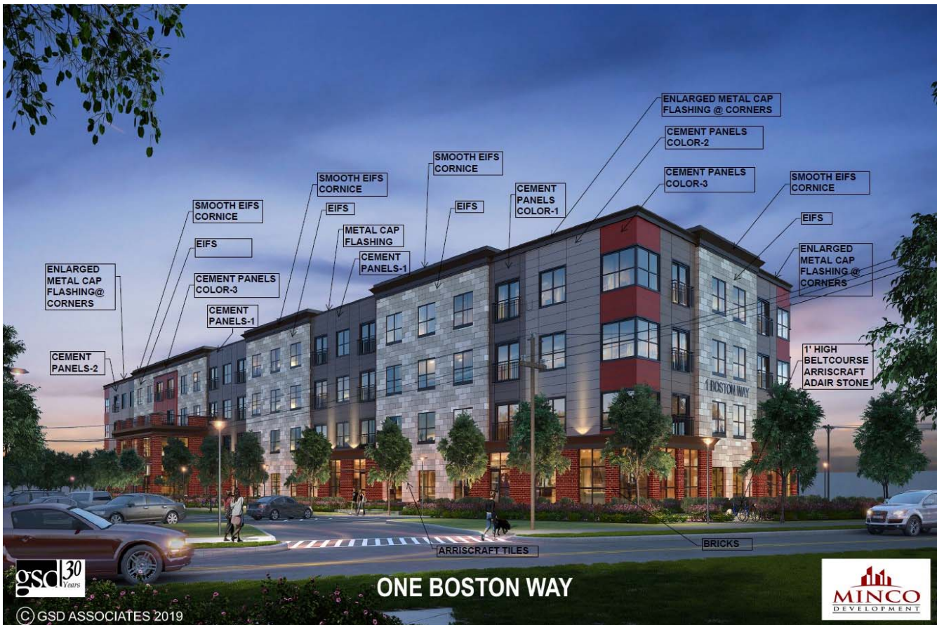
PROPOSED ELEVATION WITH MATERIALS
