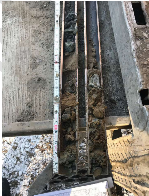
Photo 1: Split-spoon sample of silty sand and gravel from NB-1
