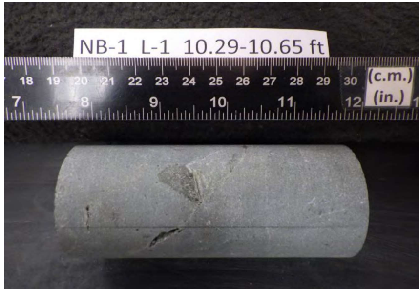
After cutting and grinding
