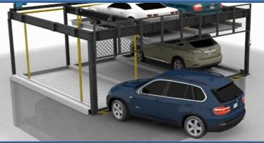
(3) Next driver retrieves car from pit space. Note blue car on right was lifted up and tan car on ground level shifted left to open up a space for the car in the pit
