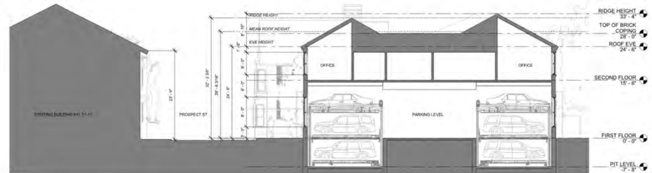
1 Prospect St Building Section 1/8" = 1'-0"
