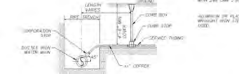
TYPICAL WATER SERVICE (NOT TO SCALE)
