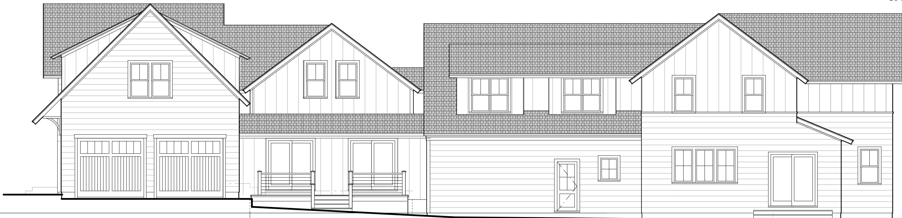
2 East Exterior Elevation - UNITS A+B SCALE: 1/8" = 1'-0"
