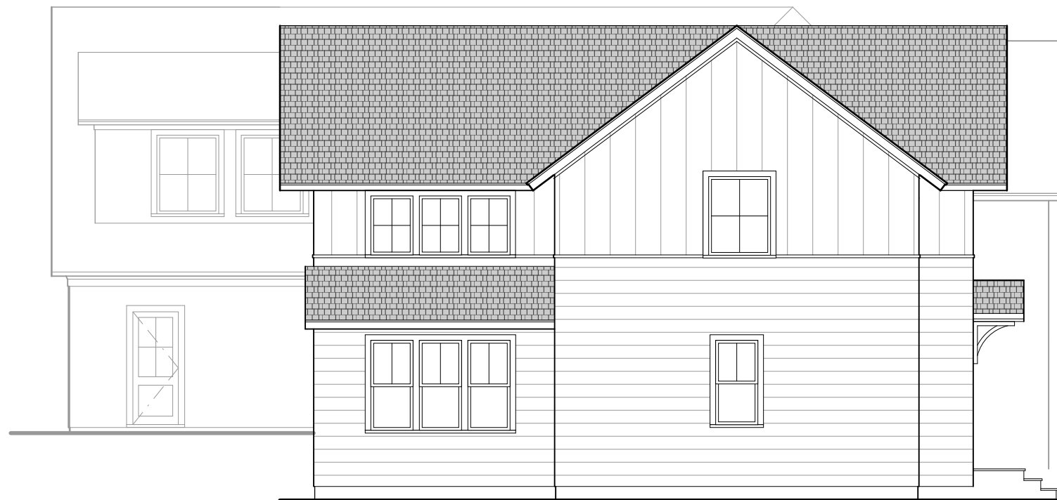
1 North Exterior Elevation - UNIT B SCALE: 1/8" = 1'-0"
