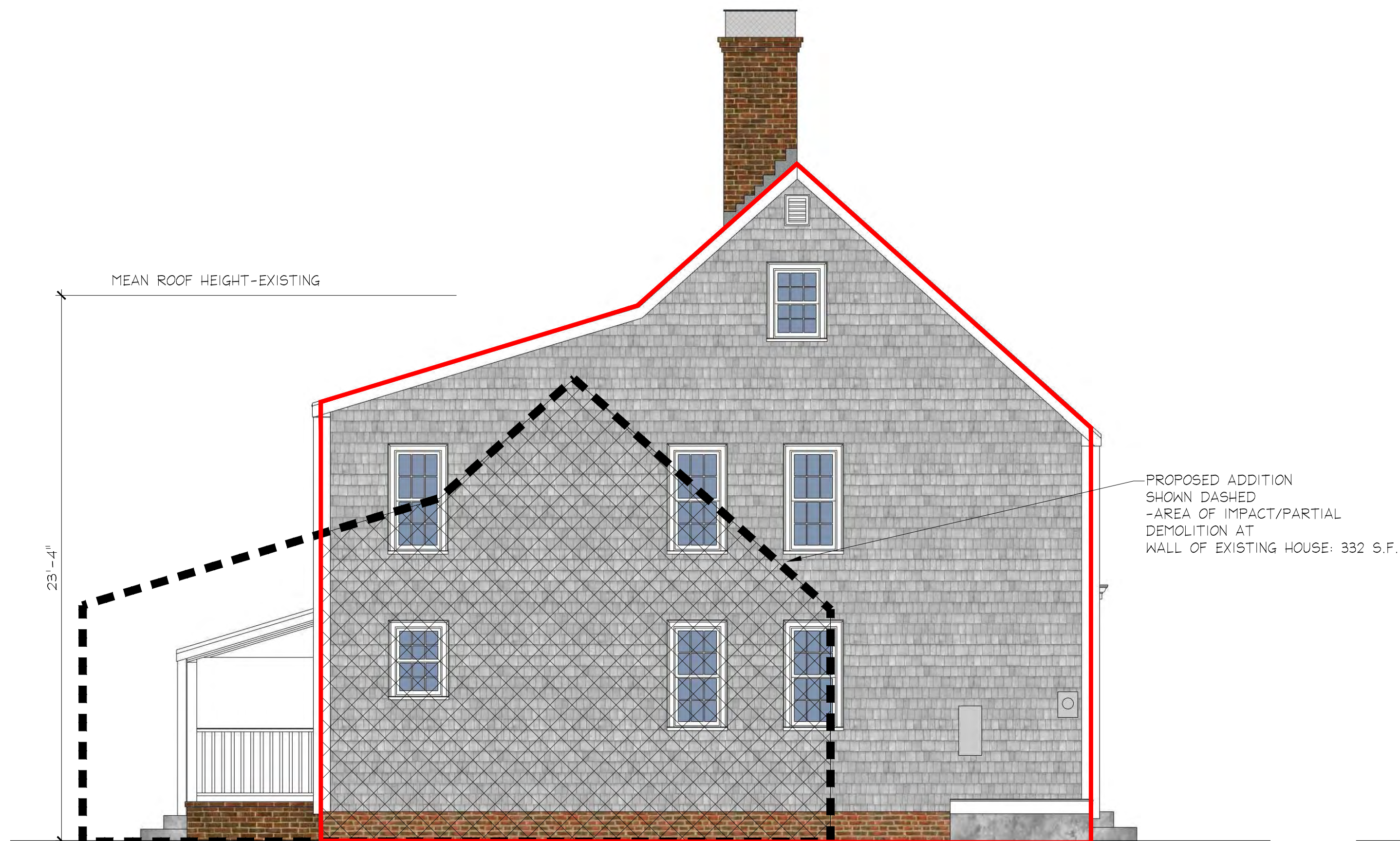
LEFT SIDE EXISTING WALL AREA: 753 S.F. OUTLINED IN RED
