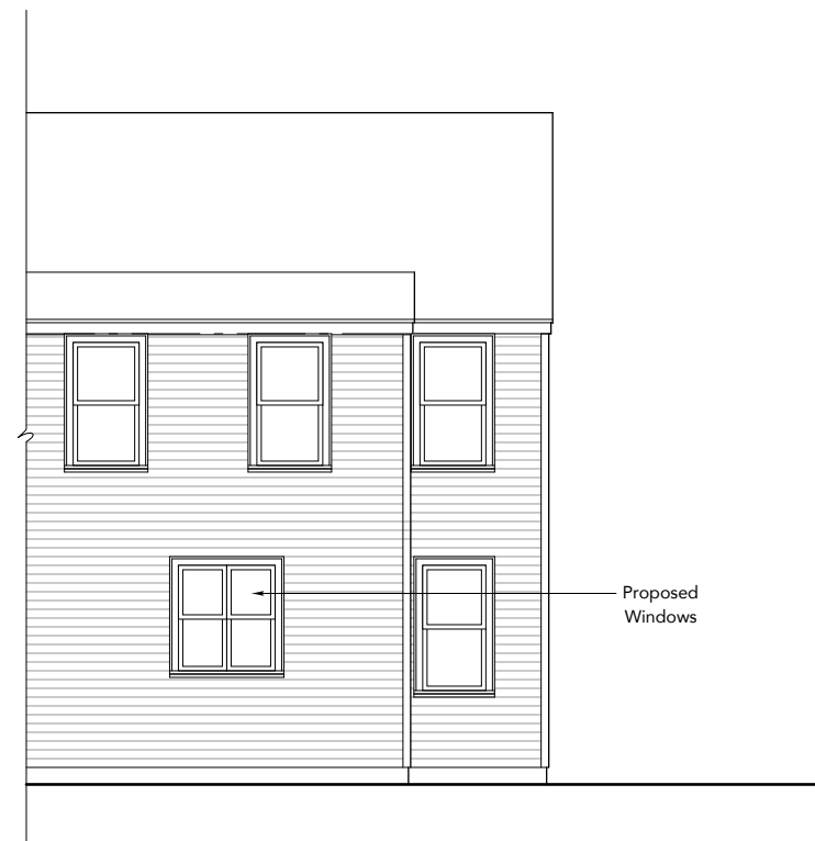
4 Rear Exterior Elevation - PROPOSED SCALE: 1/8" = 1'-0"
