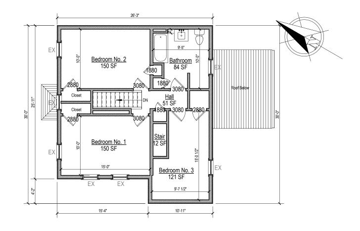
**Second Floor Plan - As-Built** Scale: 1/8" = 1'-0" 01.21.2020
