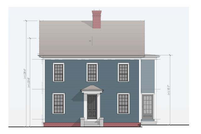
**North Elevation - As-Built** Scale: 1/8" = 1'-0" 01.21.2020
