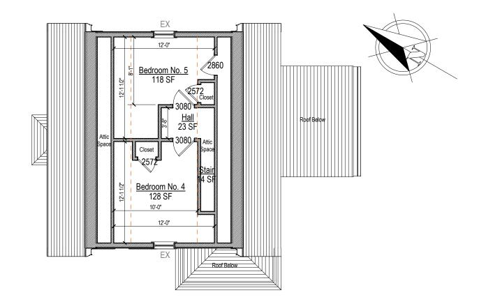
**Third Floor Plan - As-Built** Scale: 1/8" = 1'-0" 01.21.2020
