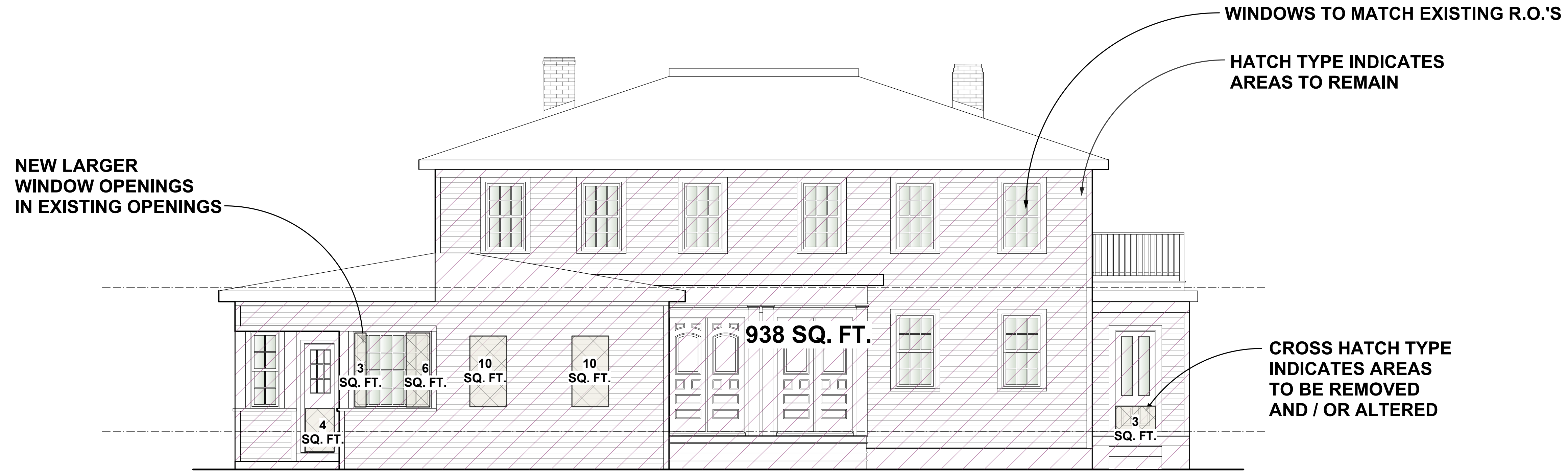
1 EXISTING FRONT ELEVATION Scale: 1/4" = 1'-0"
