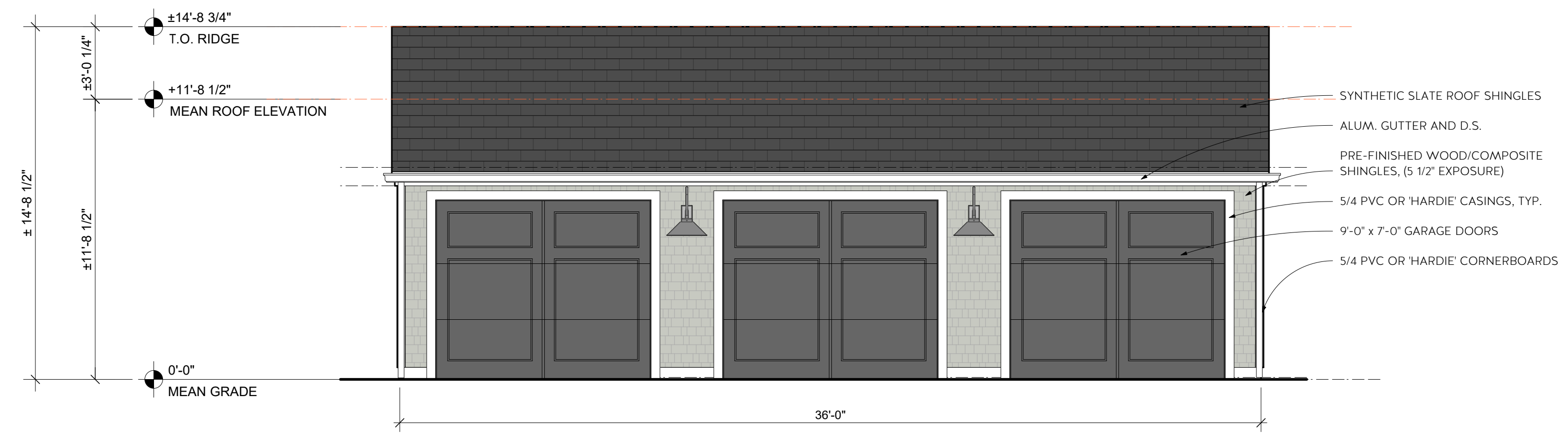
1 FRONT ELEVATION Scale: 1/4" = 1'-0"
