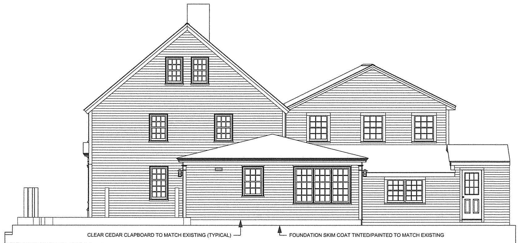
4 Proposed Southwest Elevation With Attached Neighbor Scale: 1/8" = 1'-0"
