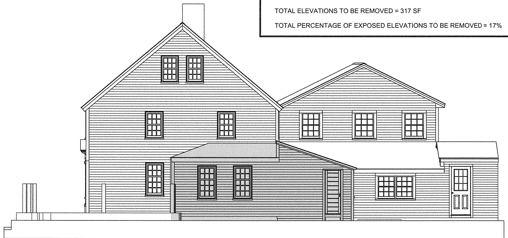
4 Existing Southwest Elevation With Attached Neighbor Scale: 1/8" = 1'-0"
