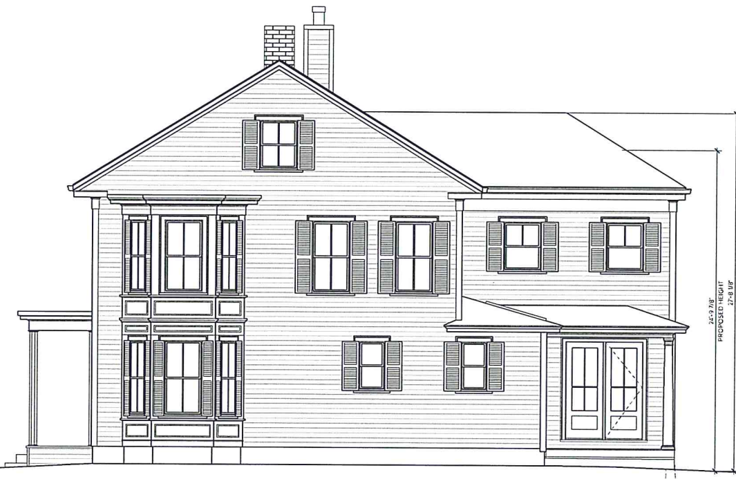
2 PROPOSED RIGHT ELEVATION Scale: 1/4" = 1'-0"
