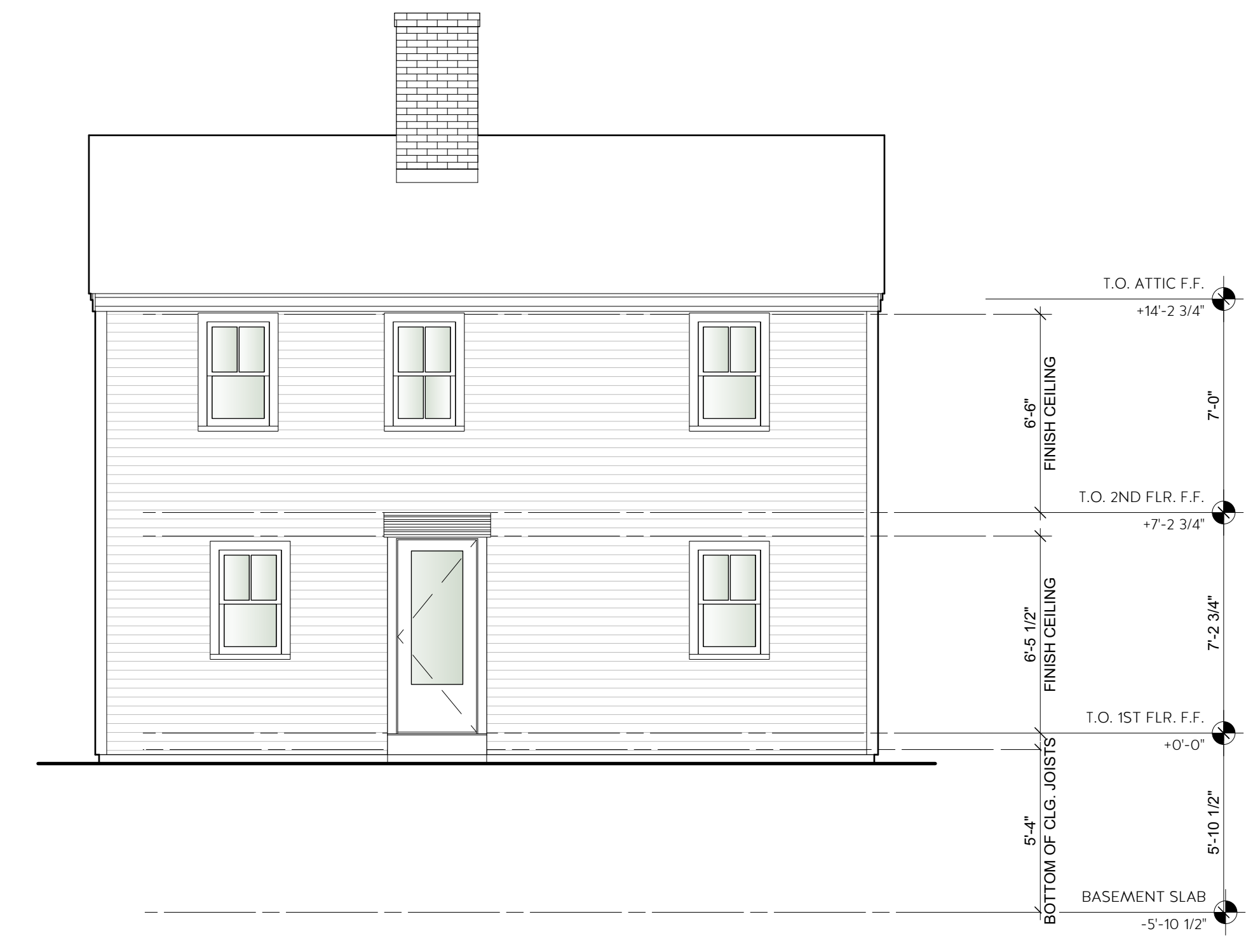
1 FRONT ELEVATION Scale: 1/4" = 1'-0"
