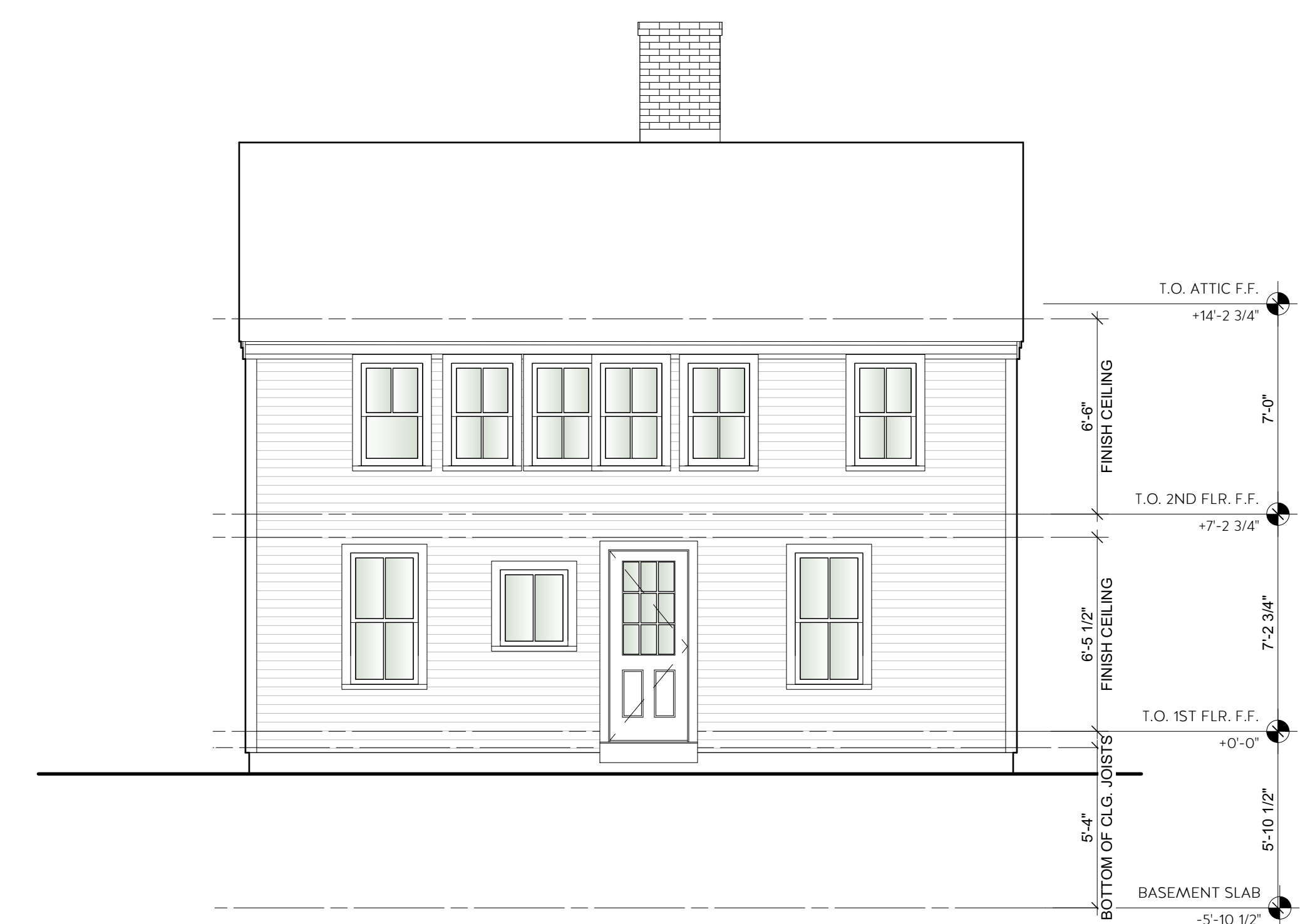
3 REAR ELEVATION Scale: 1/4" = 1'-0"
