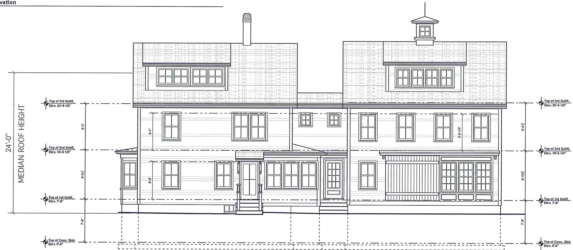
Proposed Right Side Elevation Scale: 1/4" = 1'-0"
