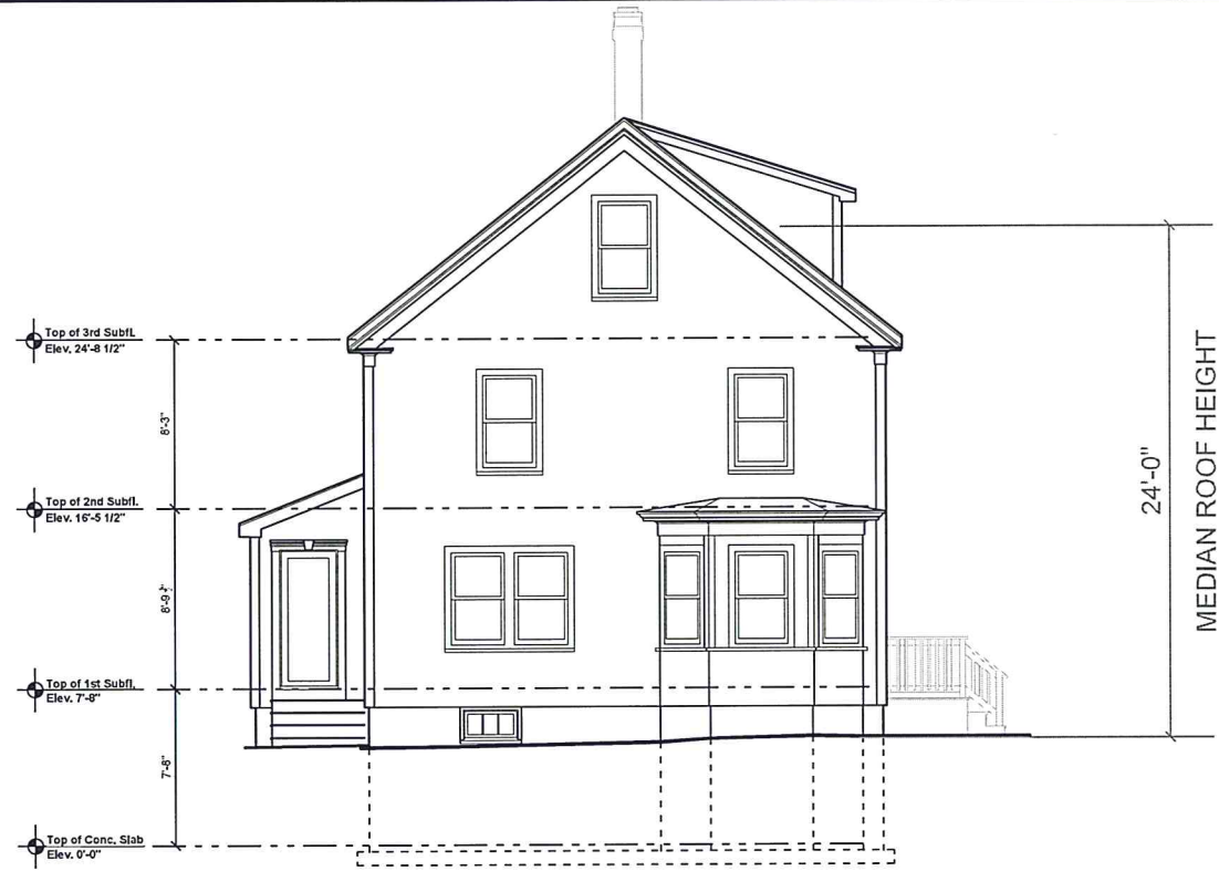
Existing Front Elevation Scale: 1/4" = 1'-0"
