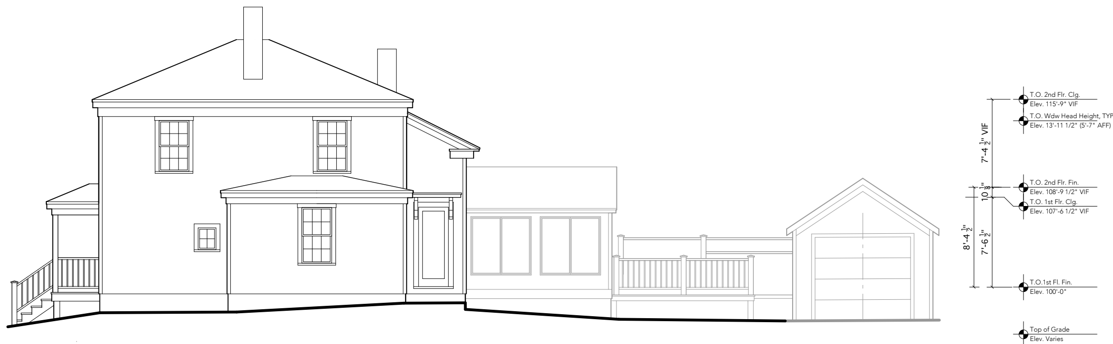
② Side (Broad Street) Exterior Elevation - EXISTING SCALE: 1/8" = 1'-0"
