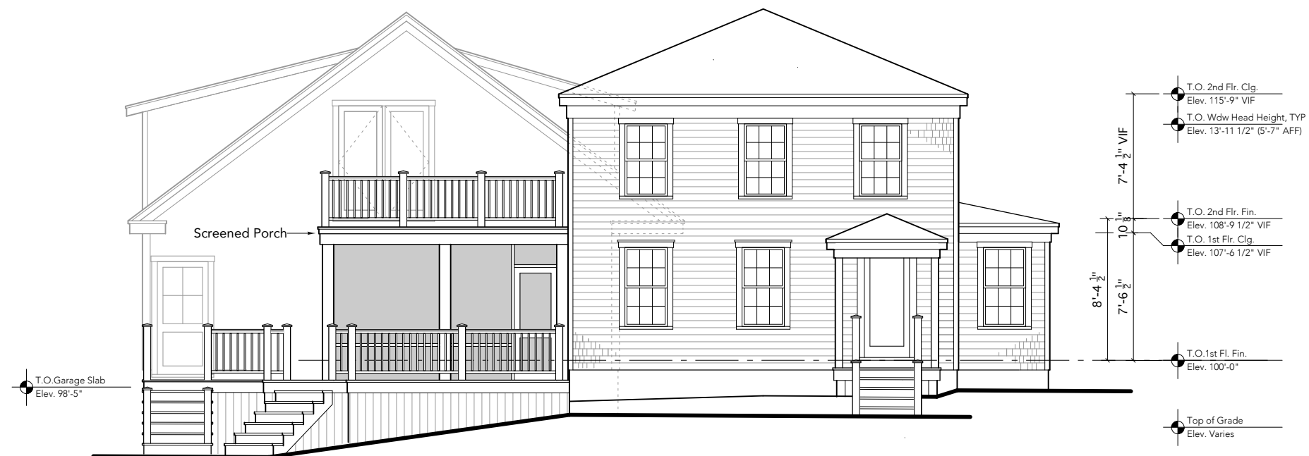
1 Front Exterior Elevation - PROPOSED SCALE: 1/8" = 1'-0"
