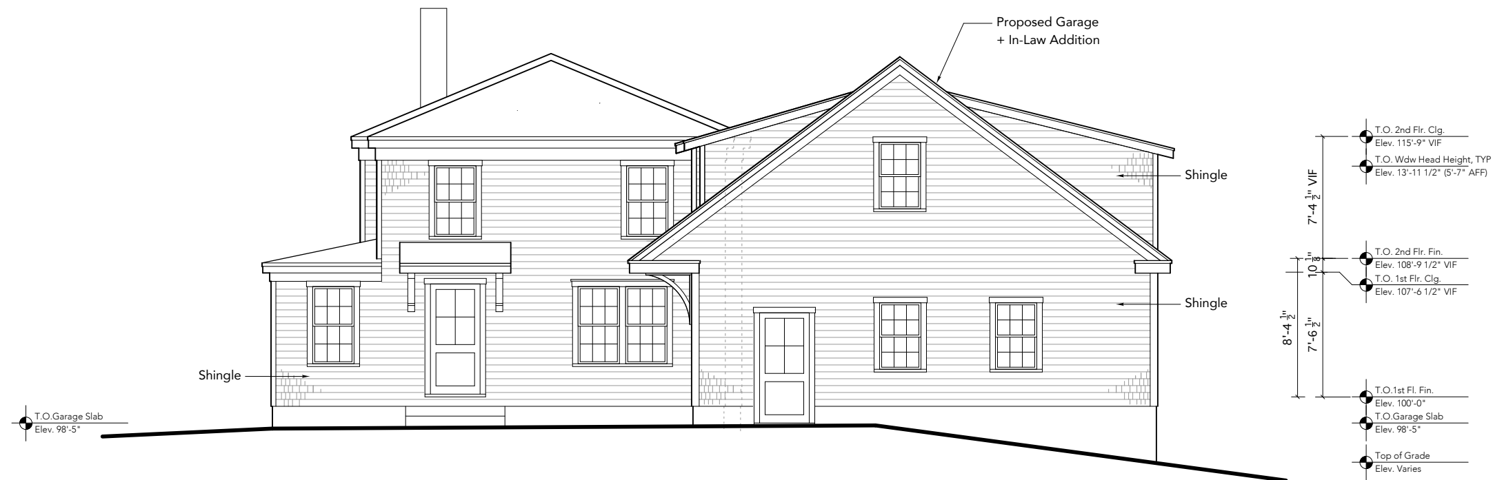
1 Rear Exterior Elevation - PROPOSED SCALE: 1/8" = 1'-0"
