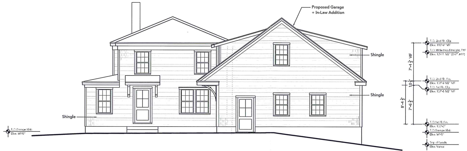
1 Front Exterior Elevation - PROPOSED SCALE: 1/8" = 1'-0"
