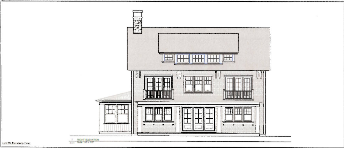
Figure 35 – Rear Elevation of the Proposed Single Family House on Beacon Ave. (Lot 1)
