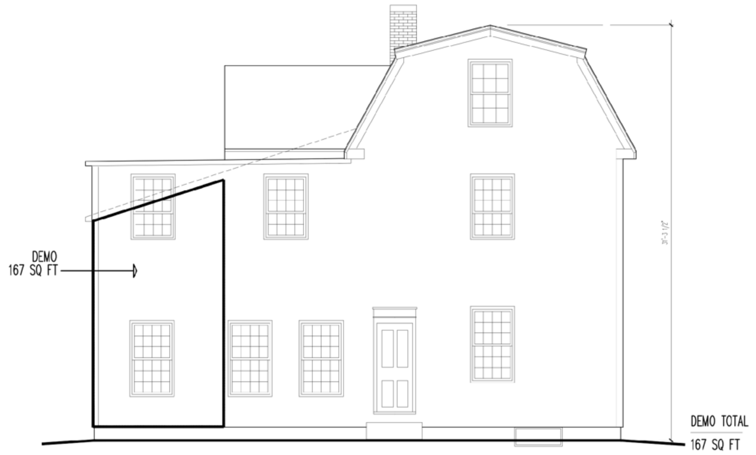
DEMOLITION LEFT SIDE ELEVATION
