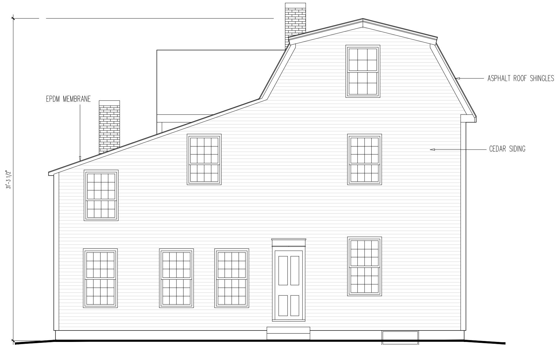
EXISTING LEFT SIDE ELEVATION
