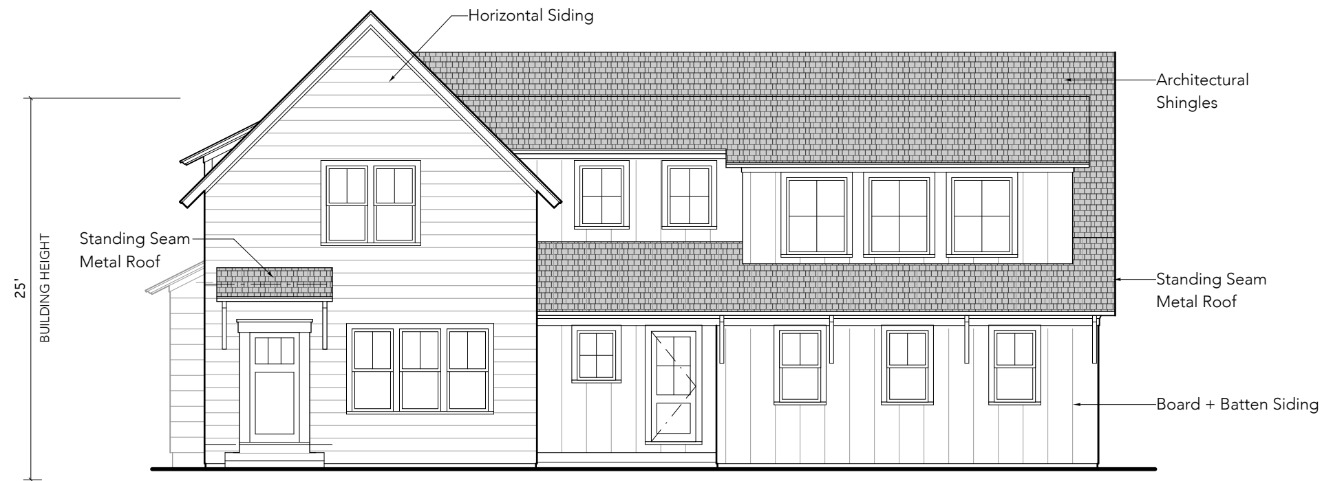
1 Exterior Elevation - UNIT A (HANCOCK ST) SCALE: 1/8" = 1'-0"
