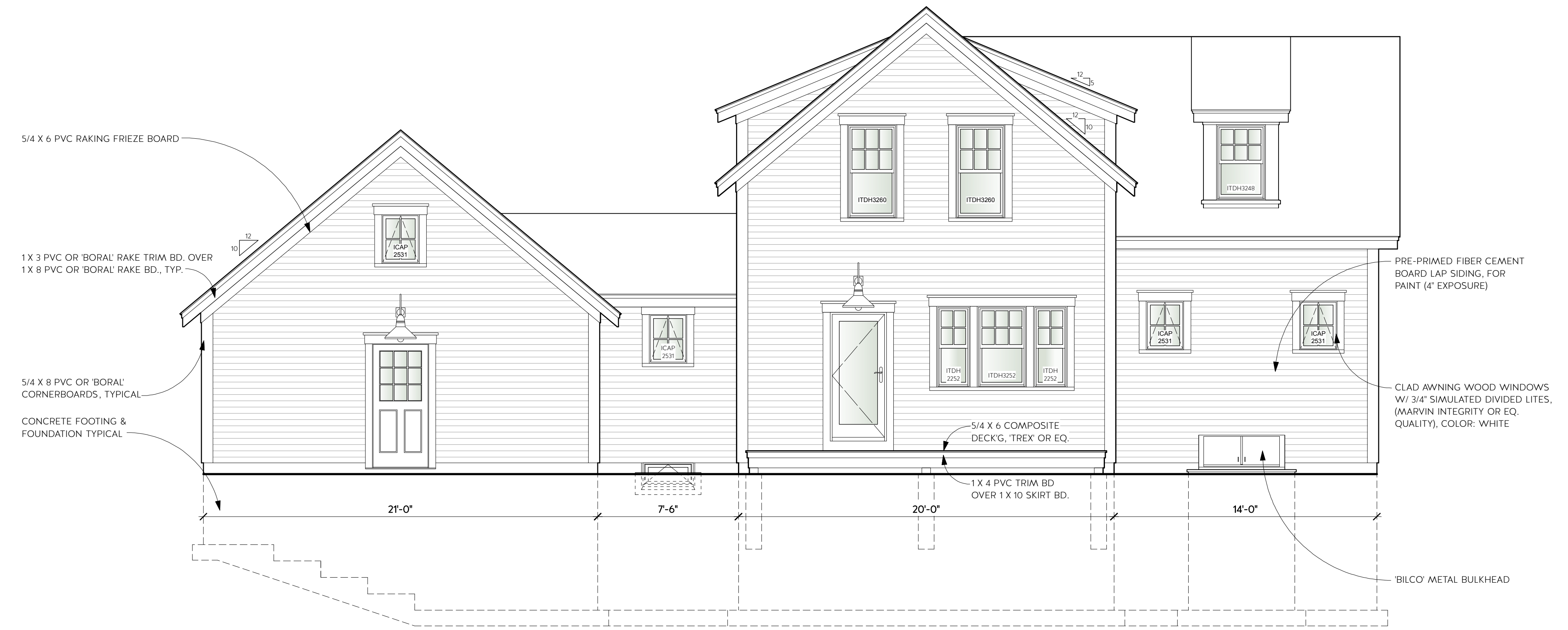
1 PROPOSED REAR ELEVATION Scale: 1/4" = 1'-0"
