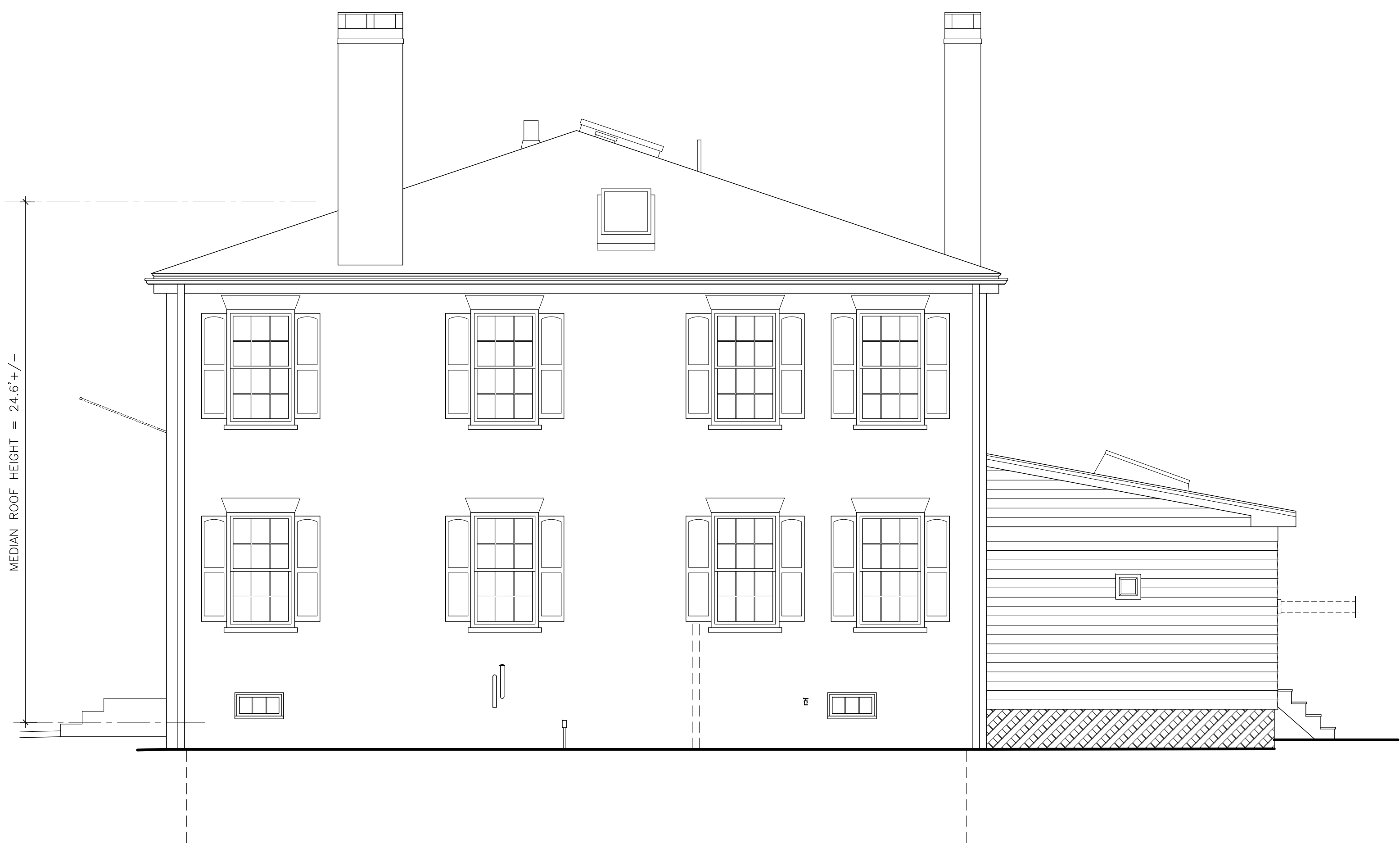
4 Existing North Elevation EX-2.0 Scale: 1/4"=1'-0"
