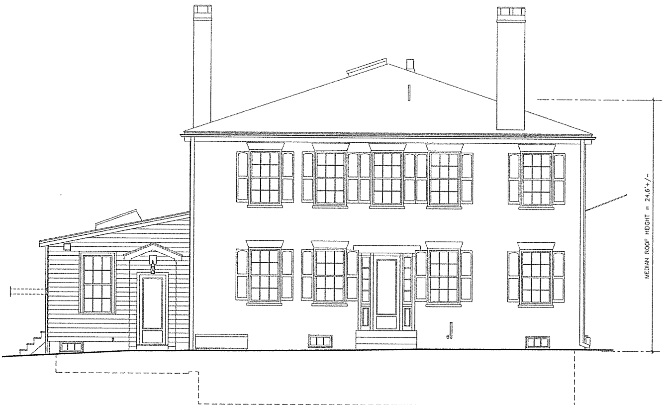
3 Existing South Elevation (Russia Street) EX-2.0 Scale: 1/4"=1'-0"
