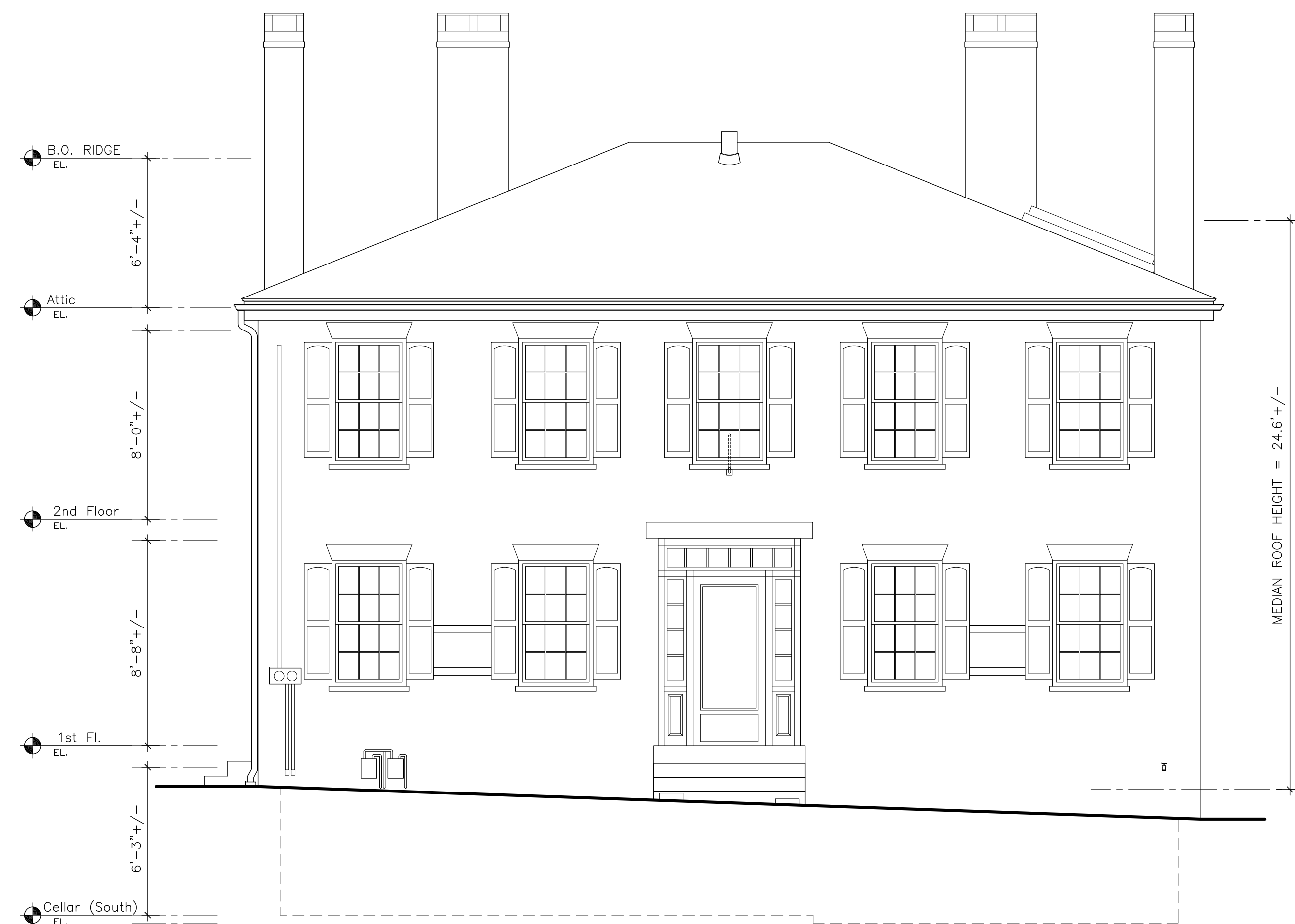
1 Existing East Elevation (Olive Street) EX-2.0 Scale: 1/4"=1'-0"
