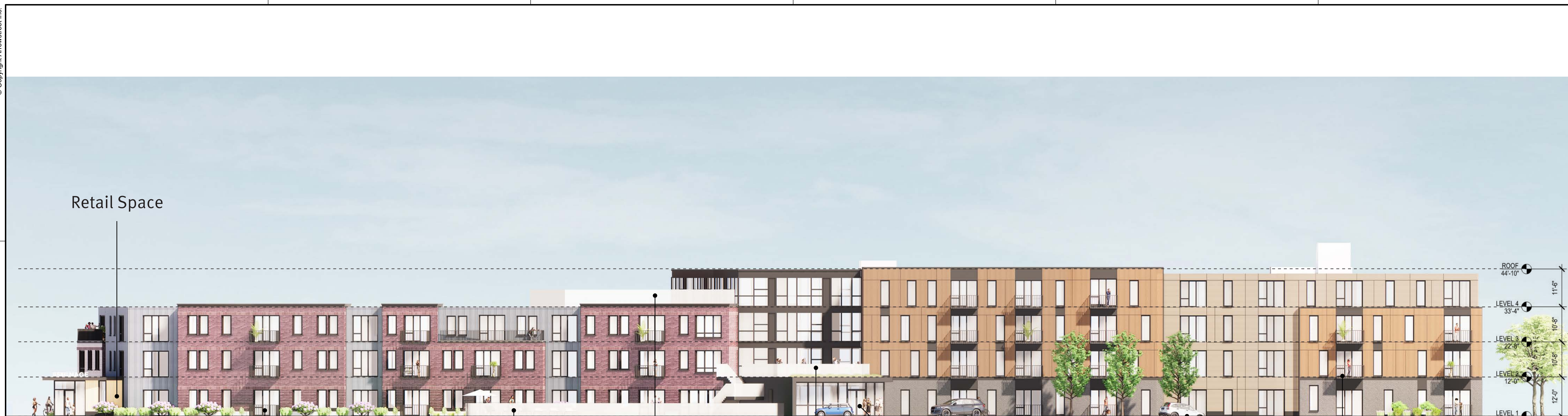
WEST ELEVATION (Clipper City Rail Trail) Retail Space Ground Floor Unit Outdoor Deck Pool & Pool Deck Fourth Floor Amenity Deck Second Floor Amenity Deck Main Entry Lobby Parking Entry Ramp Balconies ROOF 44'-10" LEVEL 4 33'-4" LEVEL 3 22'-8" LEVEL 2 12'-0" LEVEL 0 0" 11'-6" 10'-8" 10'-8" 12'-0"
