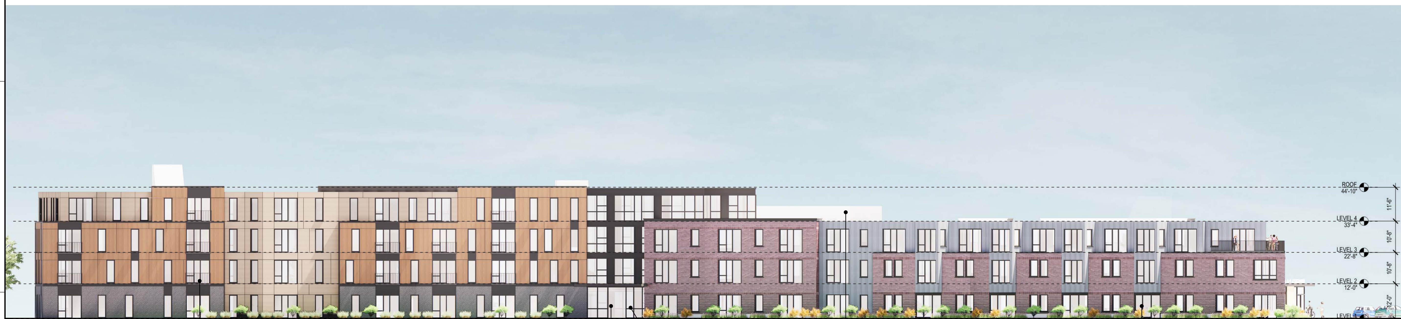
EAST ELEVATION (Route 1) Juliet Balconies Short Term Deliveries Leasing Office Fourth Floor Amenity Deck Ground Floor Unit Outdoor Deck ROOF 44'-10" LEVEL 4 33'-4" LEVEL 3 22'-8" LEVEL 2 12'-0" LEVEL 0 0" 11'-6" 10'-8" 10'-8" 12'-0"
