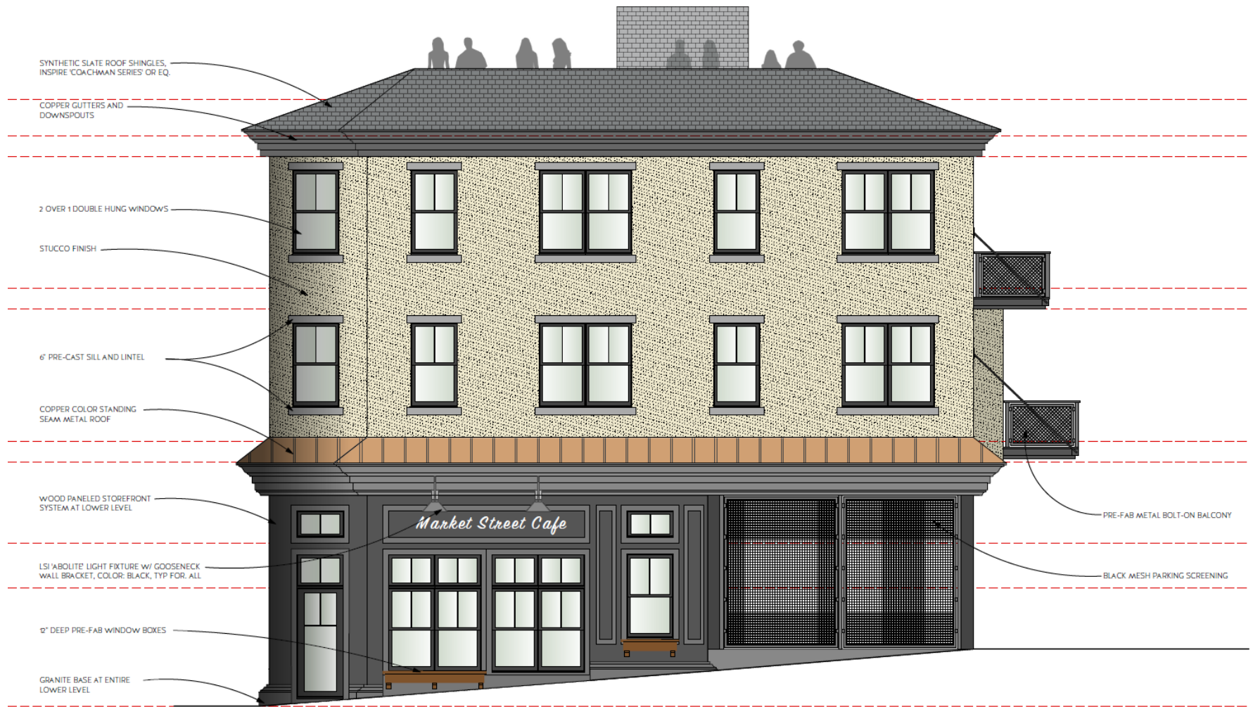
Proposed Summer Street Façade showing Building Materials
