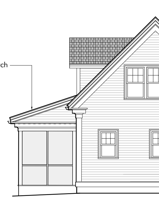
4 Exterior Elevation - SCREENED PORCH Rear SCALE: 1/8" = 1'-0"
