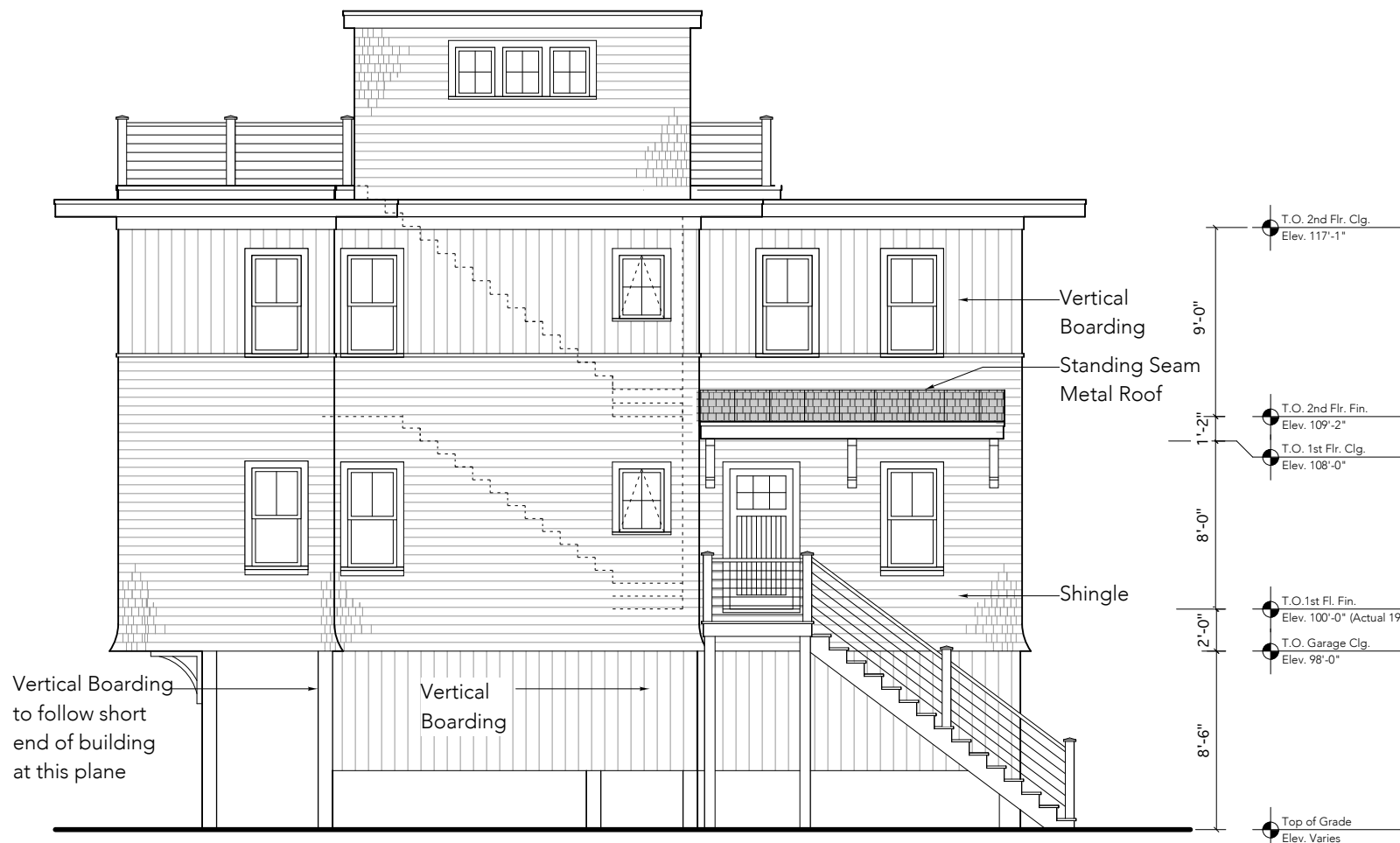
1 "Front" Exterior Elevation - Northern Blvd SCALE: 1/8" = 1'-0"
