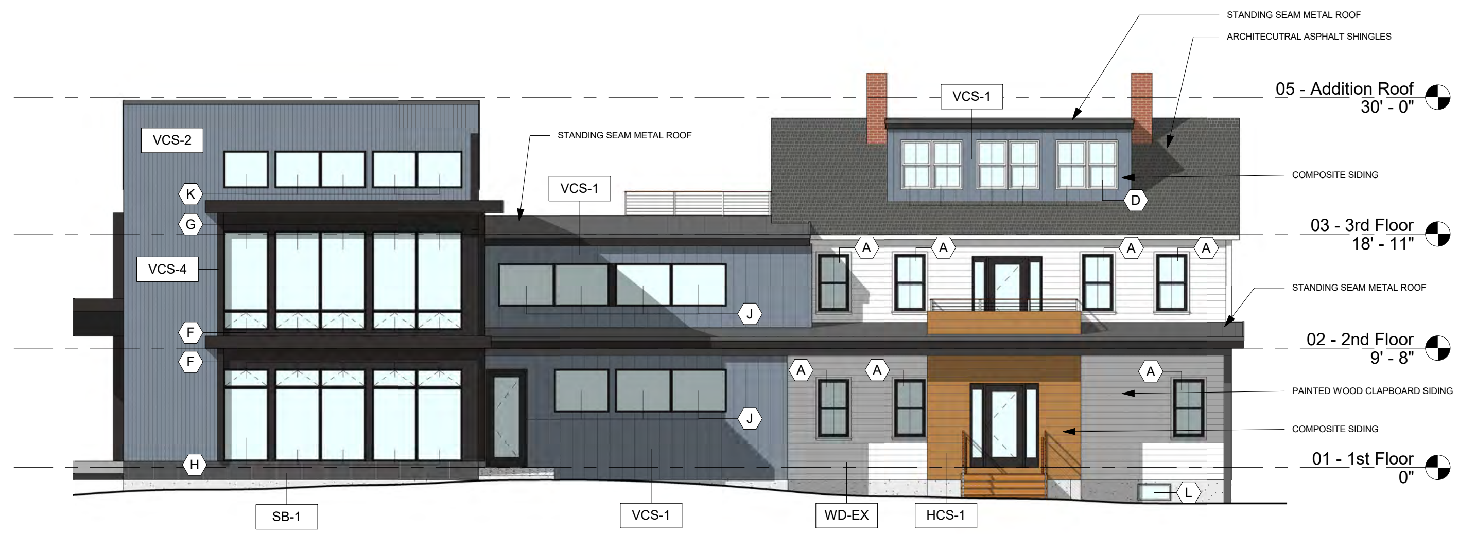
2 South Elevation - Planning Board 1/8" = 1'-0"
