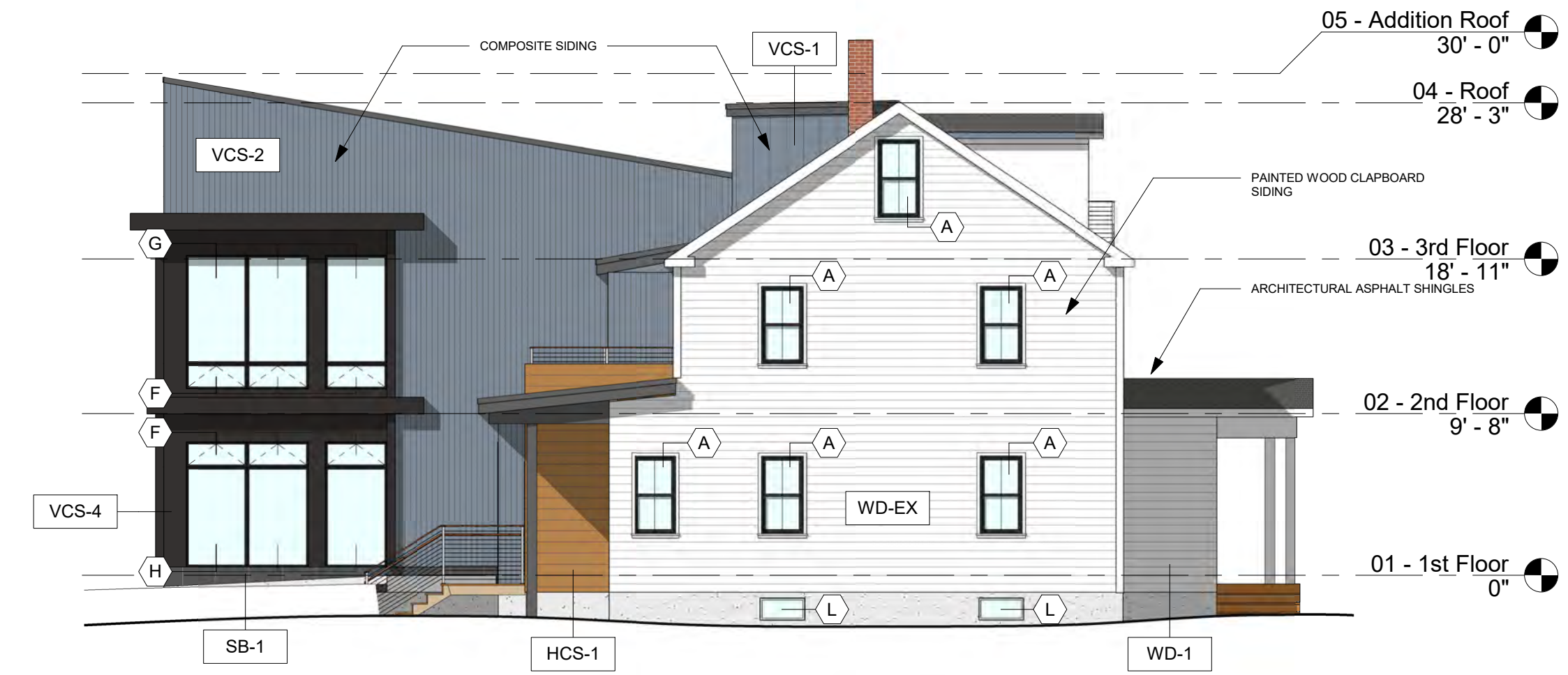
4 East Elevation - Planning Board 1/8" = 1'-0"
