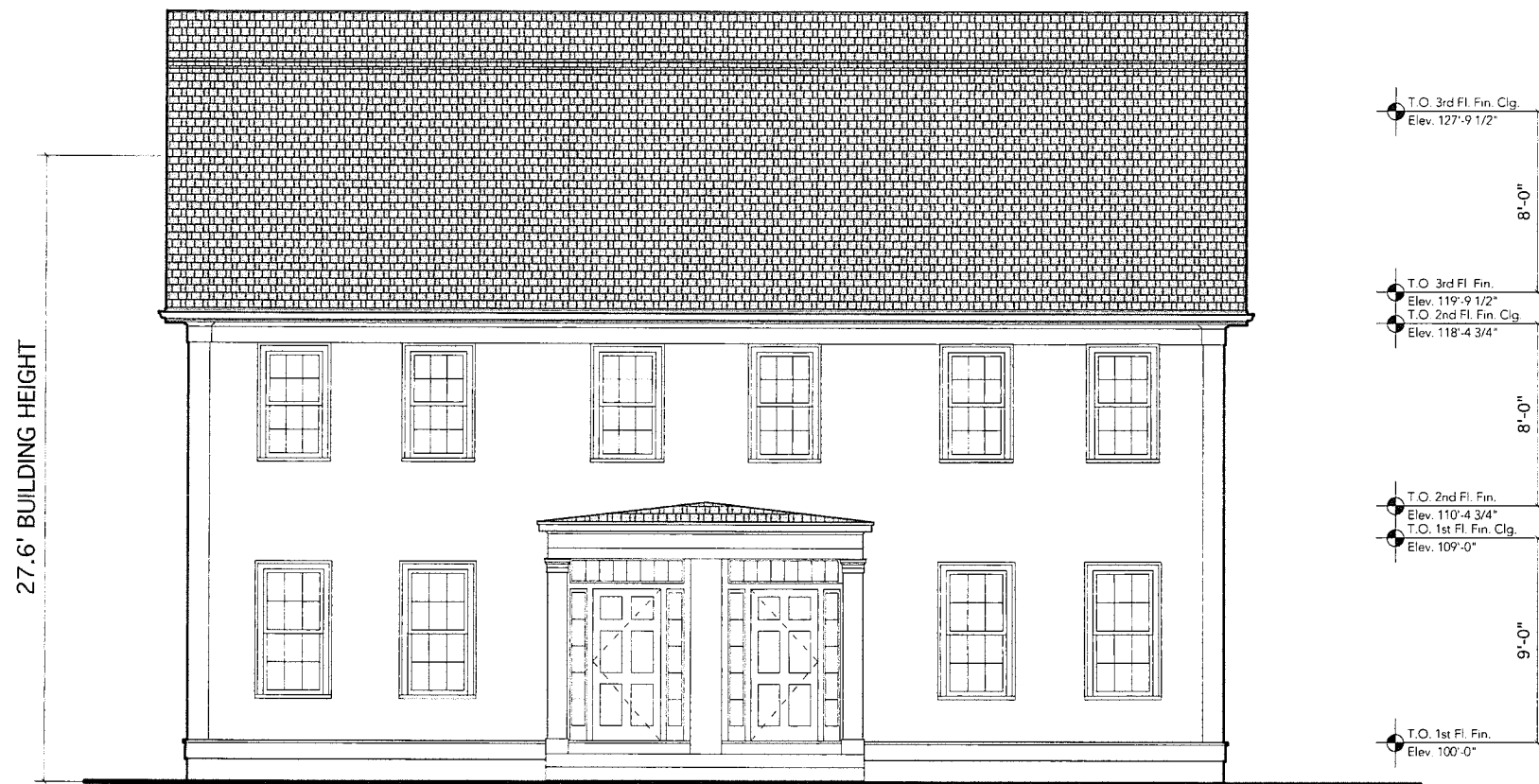
1 Exterior Elevation - Front SCALE: 1/4" = 1'-0"
