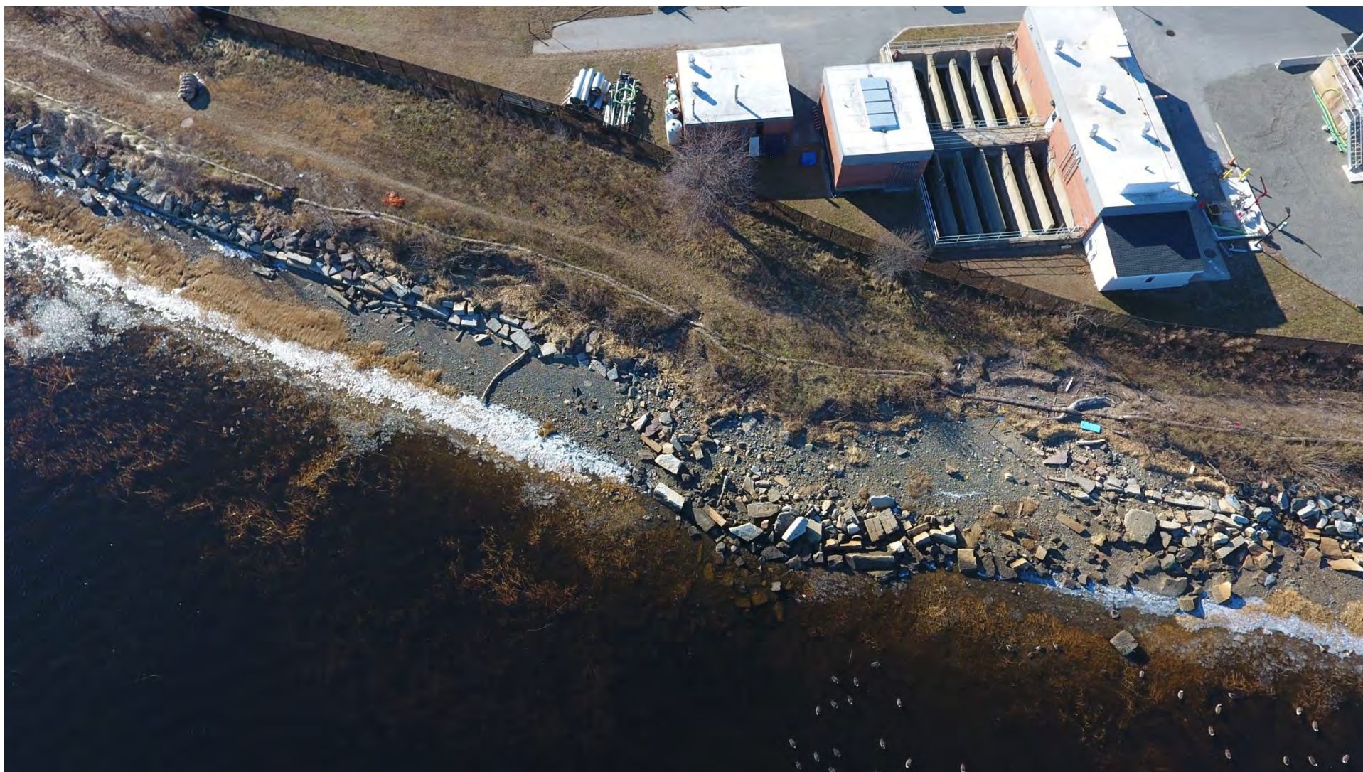
Aerial photo (December 2018) of portion of scoured shoreline along riverfront trail corridor
