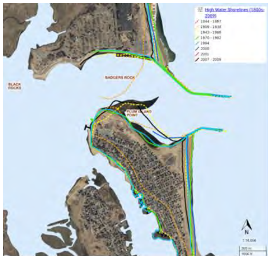
Figure 4.1.3 Map of the north and south jetties at the mouth of the Merrimack River with historic coastal edge data from 1909-2009. Source: Coastal Zone Management Massachusetts Shoreline Change Project.
