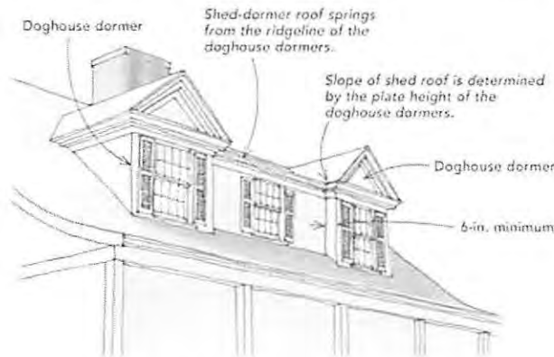
(Shed dormer with matching gabled dormers at either end)
