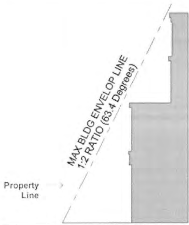
Figure 11: Upper floors must be set back from lower level building façade to ensure that taller buildings still present a comfortable and compatible scale to pedestrians.
