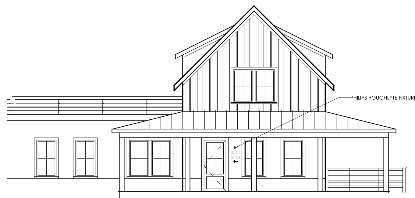
SCONCE LIGHT Front Elevation SCALE: \frac{1}{8} " = 1'-0"
