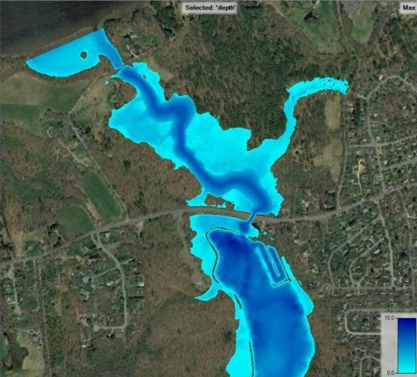
**Figure C-9:** Two Dimensional HEC-RAS Results for “Run No. 6” 100-Year frequency storm event with Mean Higher High Water (MHHW) downstream boundary conditions.
