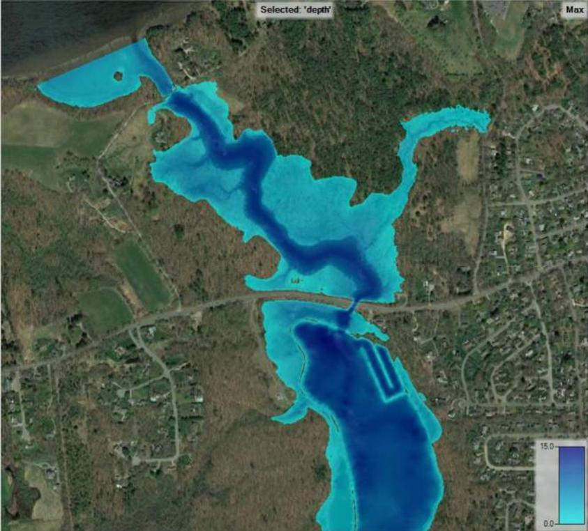
**Figure C-10:** Two Dimensional HEC-RAS Results for “Run No. 7” 500-Year frequency storm event with Mean Higher High Water (MHHW) downstream boundary conditions.
