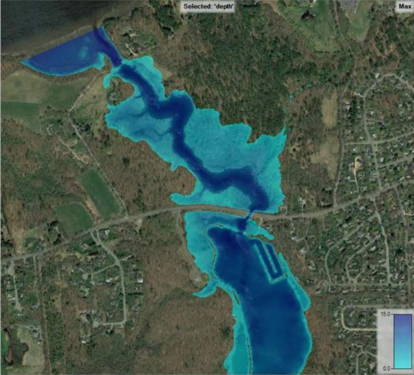
**Figure C-18:** Two Dimensional HEC-RAS Results for “Run No. 15” Merrimack River FEMA 100-Year Base Flood Elevation (BFE) downstream boundary conditions.
