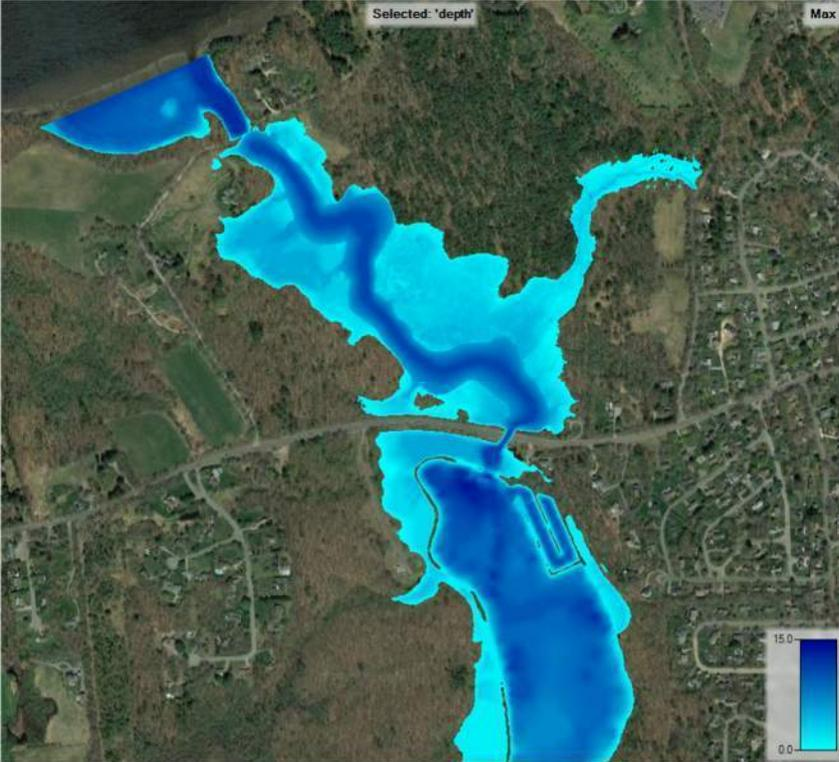
**Figure C-16:** Two Dimensional HEC-RAS Results for “Run No. 13” 100-Year frequency storm event with Mean Higher High Water (MHHW) plus Sea Level Rise (SLR) downstream boundary conditions.
