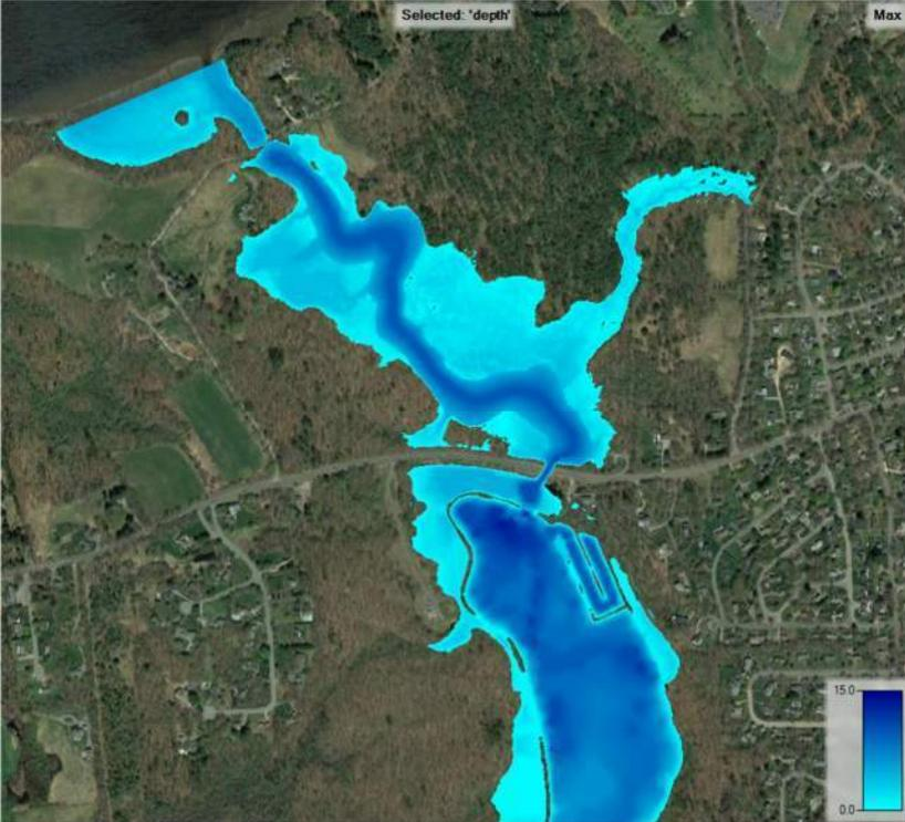
**Figure C-20:** Two Dimensional HEC-RAS Results for “Run No. 17” 50-Year frequency storm event with Mean Higher High Water (MHHW) downstream boundary conditions – Breach of Lower Artichoke Reservoir Dam.
