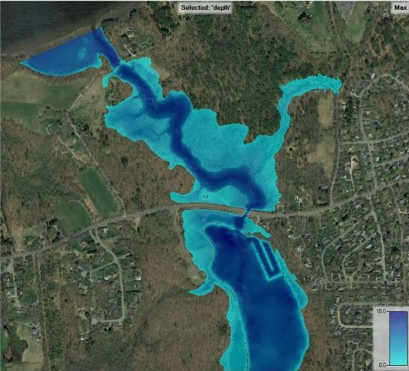
**Figure C-17:** Two Dimensional HEC-RAS Results for “Run No. 14” 500-Year frequency storm event with Mean Higher High Water (MHHW) plus Sea Level Rise (SLR) downstream boundary conditions.
