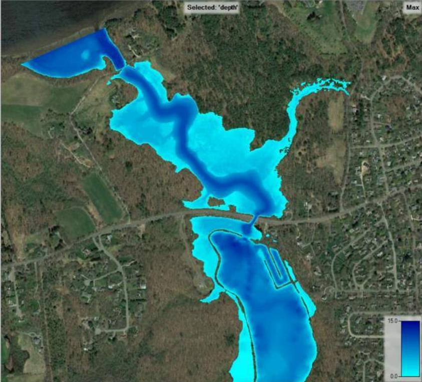
Figure C-12: Two Dimensional HEC-RAS Results for “Run No. 9” 5-Year frequency storm event with Mean Higher High Water (MHHW) plus Sea Level Rise (SLR) downstream boundary conditions.
