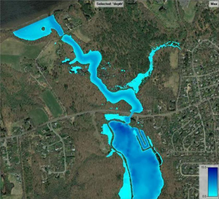
**Figure C-4:** Two Dimensional HEC-RAS Results for “Run No. 1” 2-Year frequency storm event with Mean Higher High Water (MHHW) downstream boundary conditions.
