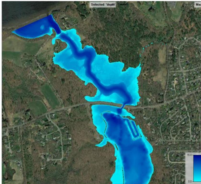
**Figure C-22:** Two Dimensional HEC-RAS Results for “Run No. 15” Merrimack River FEMA 100-Year Base Flood Elevation (BFE) downstream boundary conditions – Breach of Lower Artichoke Reservoir Dam
