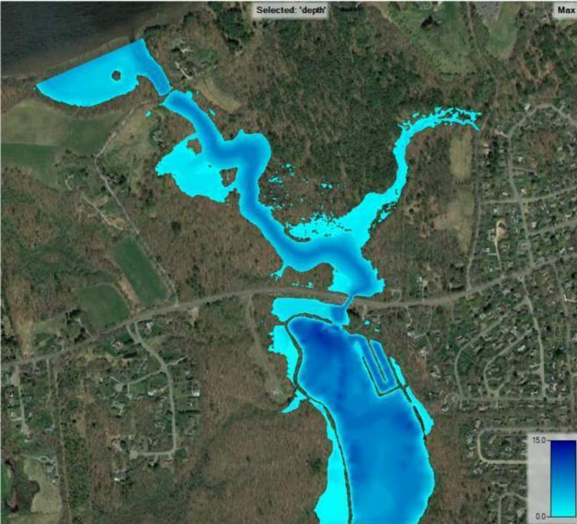
**Figure C-5:** Two Dimensional HEC-RAS Results for “Run No. 2” 5-Year frequency storm event with Mean Higher High Water (MHHW) downstream boundary conditions.
