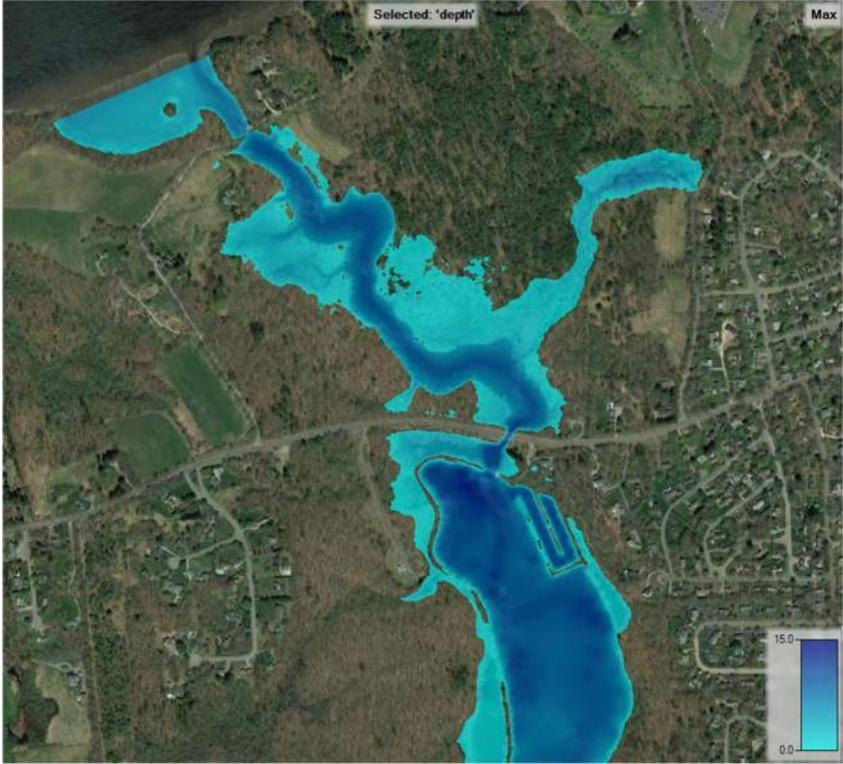
**Figure C-7:** Two Dimensional HEC-RAS Results for “Run No. 4” 25-Year frequency storm event with Mean Higher High Water (MHHW) downstream boundary conditions.
