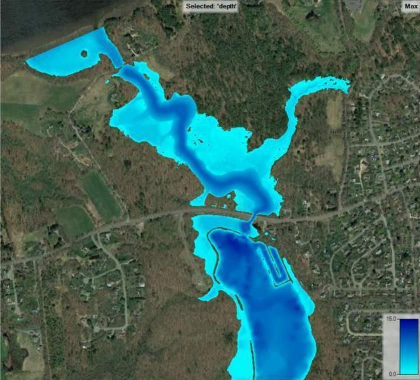
**Figure C-8:** Two Dimensional HEC-RAS Results for “Run No. 5” 50-Year frequency storm event with Mean Higher High Water (MHHW) downstream boundary conditions.
