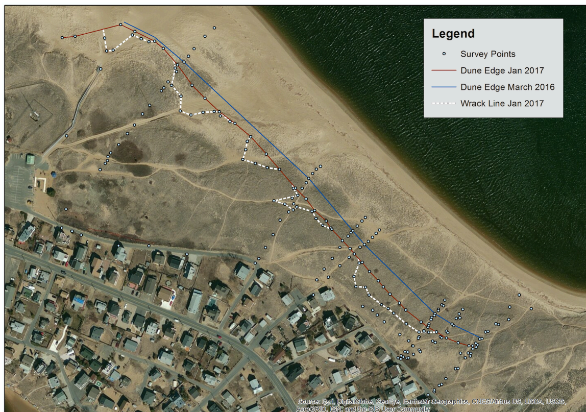
Figure 1. Leading edge of vegetated dune from March 2016 (blue line) and January 2017 (red line). The red line represents the edge of dune today, a distance of over 200ft landward of 2013 in some areas.
