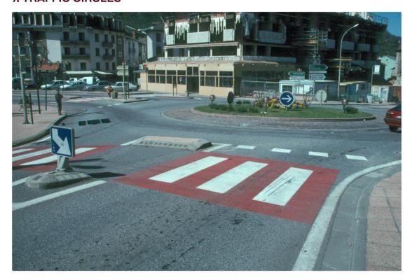
Essentially "mini-roundabouts" designed for small intersections, often used to slow traffic from a wide street into a smaller local street. Traffic circles:
